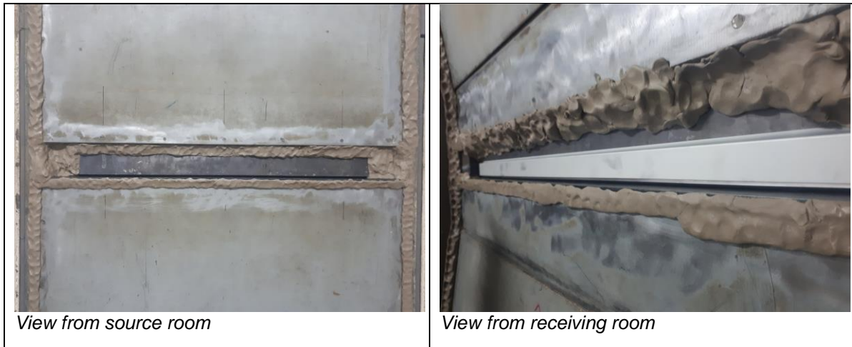
Fig. 3 Photos of the mounted element (taken by ift Laboratory for Building Acoustics)
